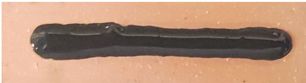
Figure S23. Optical image of the preceramic slurry deposited via extrusion-based processing onto a copper film prior to pyrolysis.
