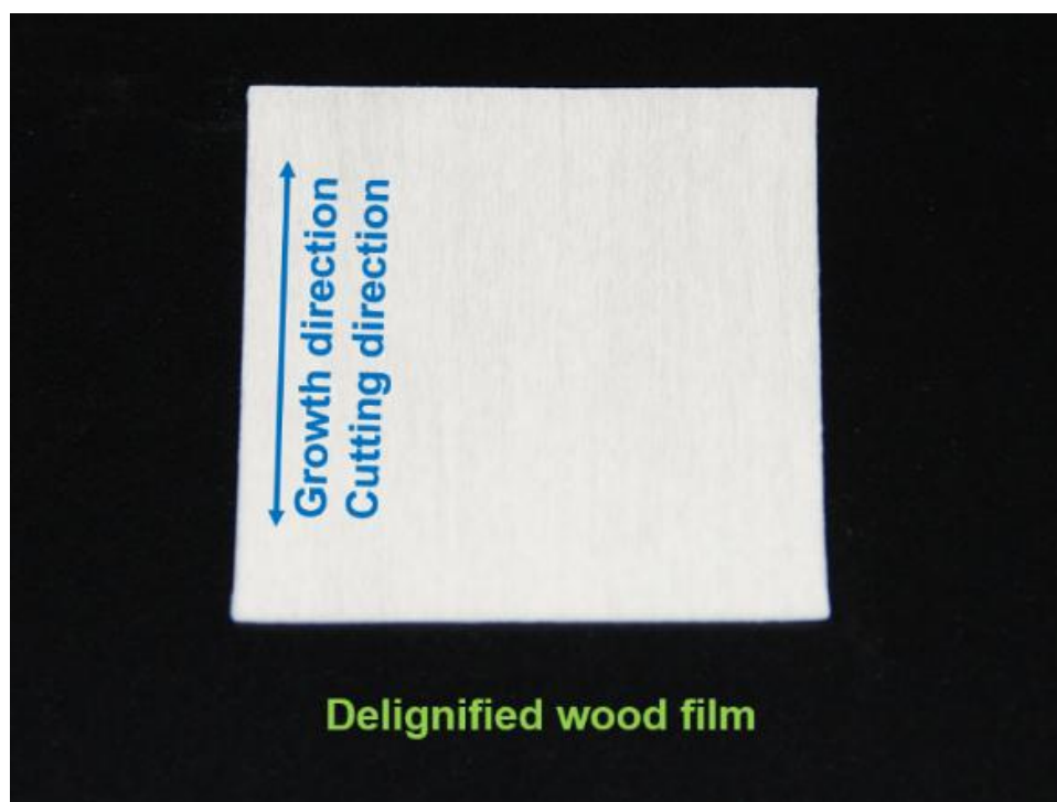
Figure S1. Delignified wood film. After delignification, the yellowish color of the natural wood was removed and the white color was obtained.
