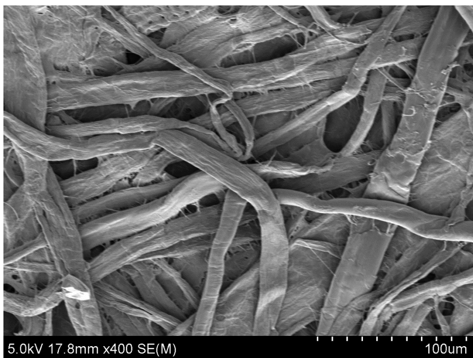
Figure S6. SEM image of filter paper. Filter paper is made of cellulose fibers, and the fibers are randomly dispersed.
