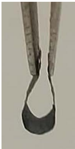
Figure S3. An optical image of a bent RGO film, demonstrating film flexibility after high temperature treatment.
