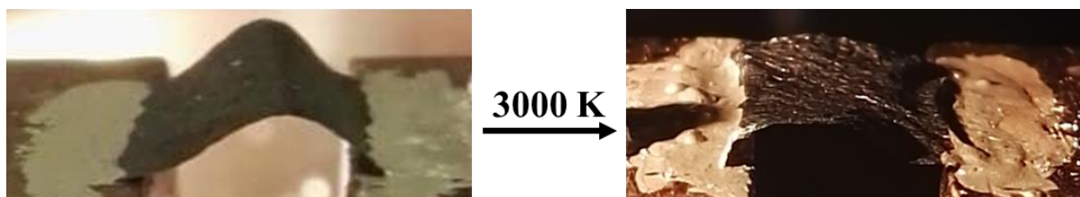
Figure S1. Pictures of the curved RGO film before and after Joule heating to 3000 K, showing that the RGO film didn't break while the degree of bending of the curved RGO film becomes smaller.
