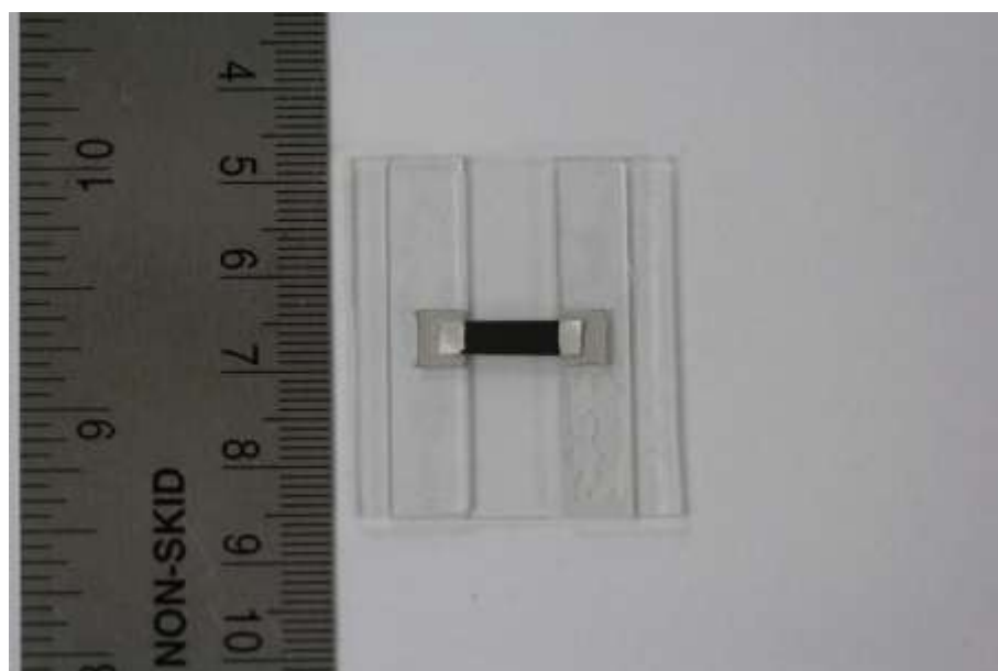
Figure S3. A typical setup for Joule heating with CSNF nanocomposite film
