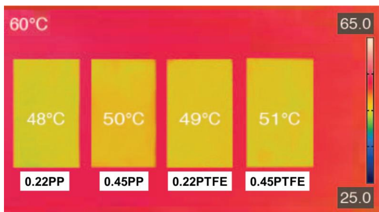
Fig. S11. IR thermographs of the commercial membranes with the heat source temperature of 60\ ^\circ\text{C} .
