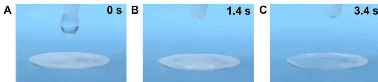
Figure S6. Snapshot photos of 2 M \text{ZnSO}_4 aqueous solution wetting ability on densified chitosan-Zn electrolyte: (A) 0 s; (B) 1.4 s; and (C) 3.4 s. The pristine chitosan-Zn membrane is semitransparent (Figure S6a). After adding a drop of \text{ZnSO}_4 aqueous solution on it, aqueous solution spreads to the whole surface of chitosan-Zn membrane quickly (Figure S6b), indicating a strong hydrophilic property. After 2 s, a transparent color in chitosan-Zn membrane is observed (Figure S6c), suggesting the aqueous solution penetrates the chitosan-Zn membrane, which also demonstrates that the aqueous solution has an excellent wetting ability to the chitosan-Zn membrane.
