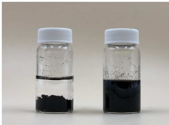
Figure S3. Photos of the CNTs dispersed in water without (left) or with (right) NFC.
