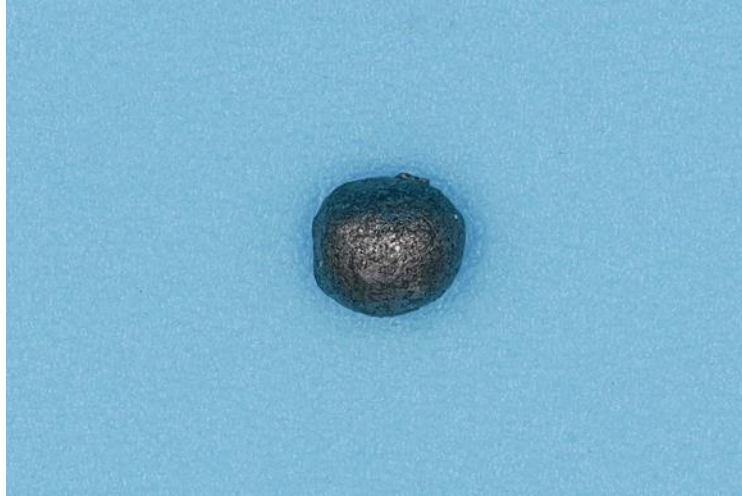
Fig. S4. Sample morphology. The HEB composite melts, loses its original geometry and becomes a spherical ingot, when the heating treatment temperature is \sim 3300 K.
