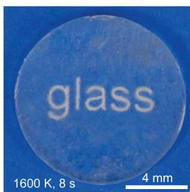
Figure S16. Optical image of the sintered silica glass at \approx 1600 K with a sintering holding time of 8 s.
