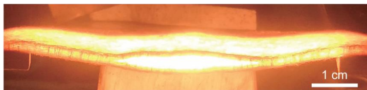
Figure S4. Optical image of the carbon heater during the UHS process at \approx 1600 K.
