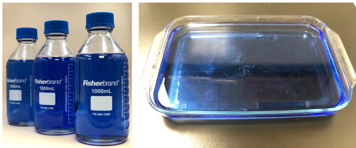
Supplementary Fig. 22: Cu(II)-saturated NaOH solution (at a NaOH concentration of 10 wt%). As an example, 3 L of Cu(II)-saturated NaOH solution can be prepared within 1 day. The process is easy to scale up and NaOH can be recycled from the waste solution (Fig. 5a).
